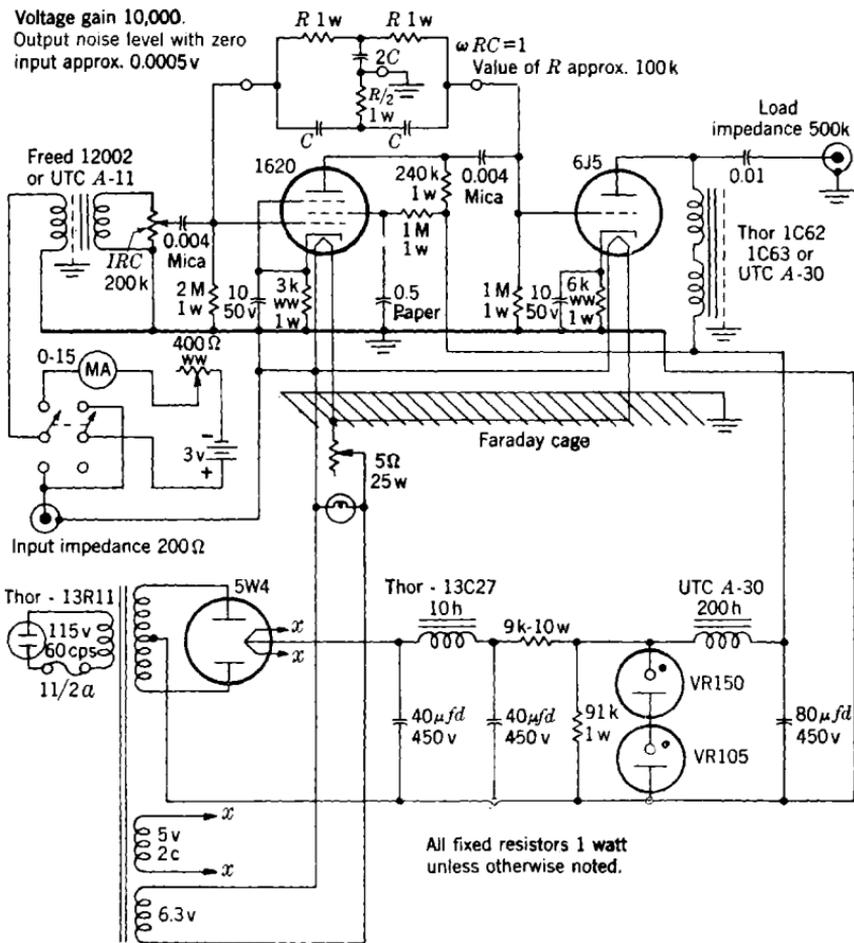
Fig. 16-12. Tuned audio amplifier.
