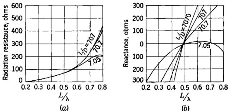
FIG. 8-8.—Input impedance of spheroidal dipoles with major axis  $L$  and minor axis  $D$ : (a) real component or radiation resistance; (b) imaginary component or reactance. (From *L. J. Chu and J. A. Stratton, J. Appl. Physics*, by courtesy of the authors and the American Institute of Physics.)
