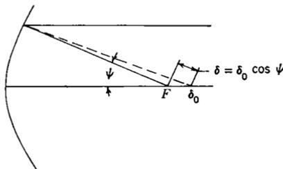
FIG. 12-7.—Defocusing phase errors.
