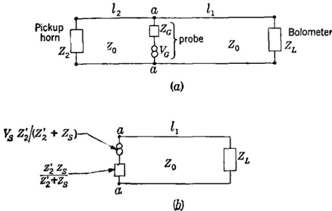
FIG. 15-12.—Equivalent circuit of r-f probe.
