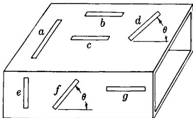
FIG. 9-16.—Slots in the wall of rectangular waveguide.
