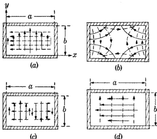
FIG. 7-9.— $TE$ -modes in rectangular waveguides: (a)  $TE_{10}$ -mode [ $\lambda_{10}^{(c)} = 2a$ ]; (b)  $TE_{11}$ -mode [ $\lambda_{11}^{(c)} = 2ab/\sqrt{a^2 + b^2}$ ]; (c)  $TE_{20}$ -mode [ $\lambda_{20}^{(c)} = a$ ]; (d)  $TE_{01}$ -mode ( $\lambda_{01}^{(c)} = 2b$ ). ——— electric field; - - - - magnetic field.
