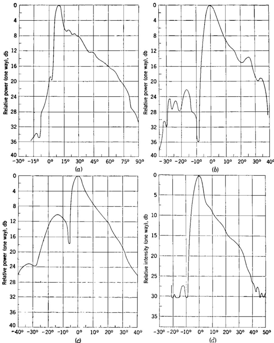
FIG. 13-20.—Elevation patterns obtained with airborne shaped-reflector antennas: (a) barrel-reflector antenna of Fig. 13-17; (b) shovel-reflector antenna of Fig. 13-18; (c) strip-reflector antenna of Fig. 13-19; (d) cut-down barrel-reflector antenna.
