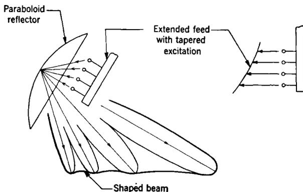
FIG. 13-8.—Formation of a shaped beam by means of a feed array in a paraboloid reflector. process; the rays emerging from the aperture will not all be collimated but will be distributed through a range of angles with a variable density dependent upon the pattern required. Defocusing in one plane can be accomplished either by extending the point source into a line source in that plane or by modifying the reflector or lens in that plane.
