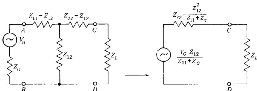
FIG. 2-4.—Thévenin's theorem and the maximum-power transfer condition.
