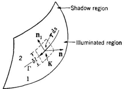
FIG. 5-7.—Calculation of the electric charge on the shadow boundary curve  $\Gamma$ .
