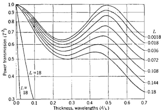
Fig. 14-14. Power transmission  $|T|^2$  as a function of thickness for various values of loss tangent  $L = \epsilon''/\epsilon'$ .
