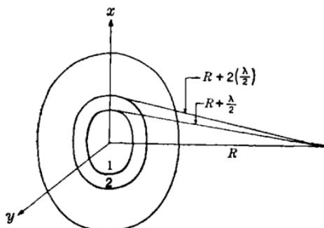
FIG. 6-9.—Division of the aperture into Fresnel zones.
