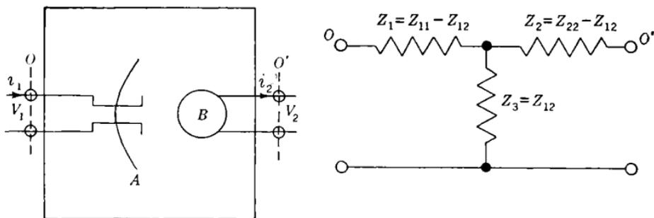
FIG. 2.11.—Four-terminal network representation of the coupled transmitter-receiver.
