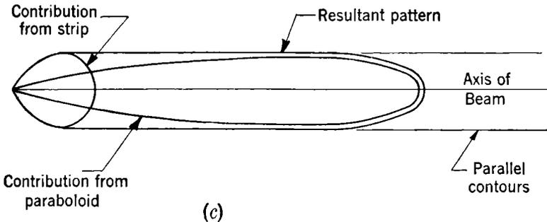
out strip; (b) central horizontal section showing strip; (c) mechanism of beam shaping.
