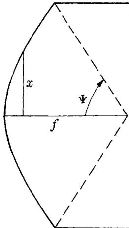
FIG. 12-29.—A pillbox of angular aperture  $\Psi$ .
