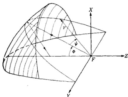
FIG. 13-33.—Double curvature surface and spherical coordinate system.
