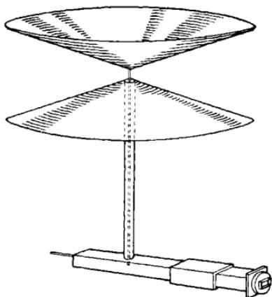
FIG. 1-3.—The biconical horn.
