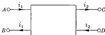
FIG. 2-1.—Four-terminal network.
