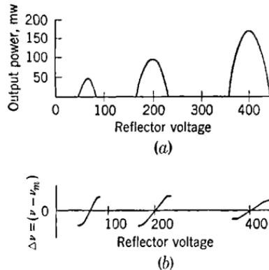
FIG. 16-2.—Operating characteristics of a reflex klystron: (a) variation in output r-f power with voltage; (b) change in output frequency with respect to the frequency  $\nu_m$  of the maximum power of the mode.
