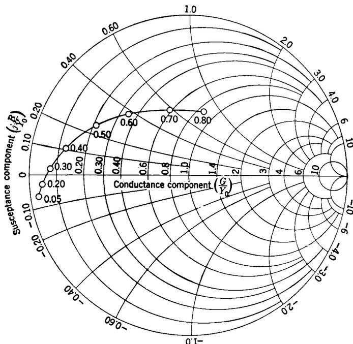
FIG. 9-15.—Dipole admittance as a function of probe depth in inches ( $\lambda = 10.7$  cm).
