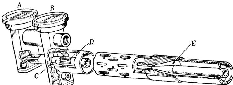
FIG. 9-54.—Double antenna system,  $\lambda = 3$  cm.
