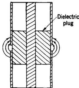
FIG. 9-35.—Longitudinally polarized slot radiator for coaxial line.
