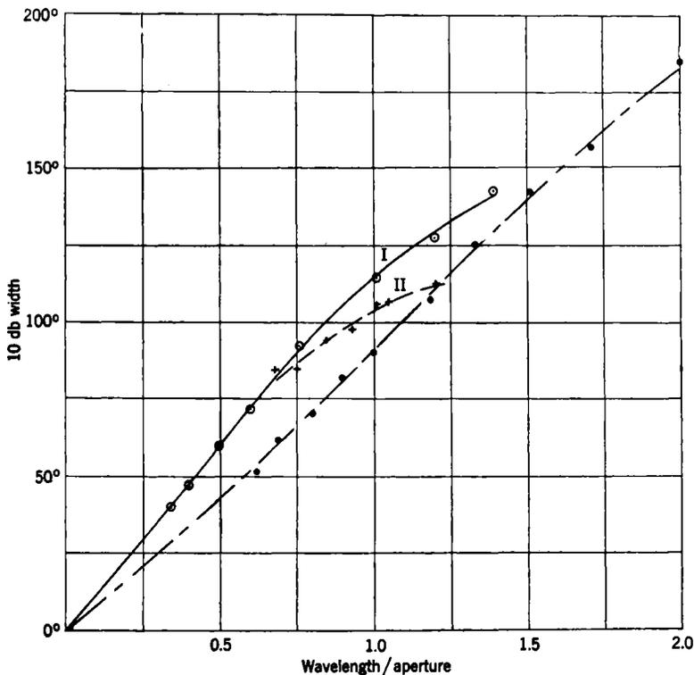
FIG. 10-15.—Experimental 10-db widths of horns having small phase variations over the aperture ( $\frac{\delta}{\lambda_0} < \frac{1}{8}$ ). ———— *E*-plane; - - - - - *H*-plane sectoral horns; ——— *H*-plane of compound horns with *E*-plane aperture equal to or greater than a wavelength.
