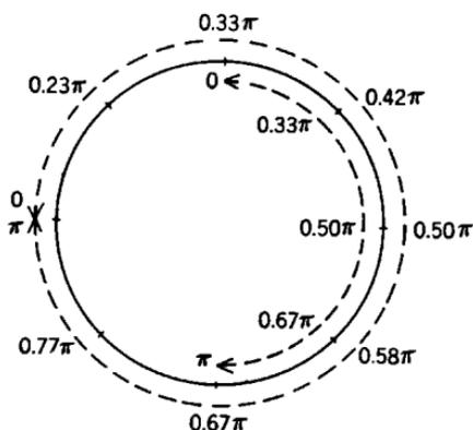
FIG. 9-9.—The range of  $\psi$ , the angle of  $z$ , as  $\theta$  varies from 0 to  $\pi$ . The outer ring of figures shows corresponding values of  $\theta$  at various points on the unit circle in the  $z$ -plane for  $s = \lambda/2$ . The inner set of figures shows values of  $\theta$  for  $s = \lambda/4$ .
