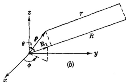
FIG. 3-5.—On the far-zone field: (a) arbitrary field point  $P$ ; (b) simplifying relationships for a point in the far zone.
