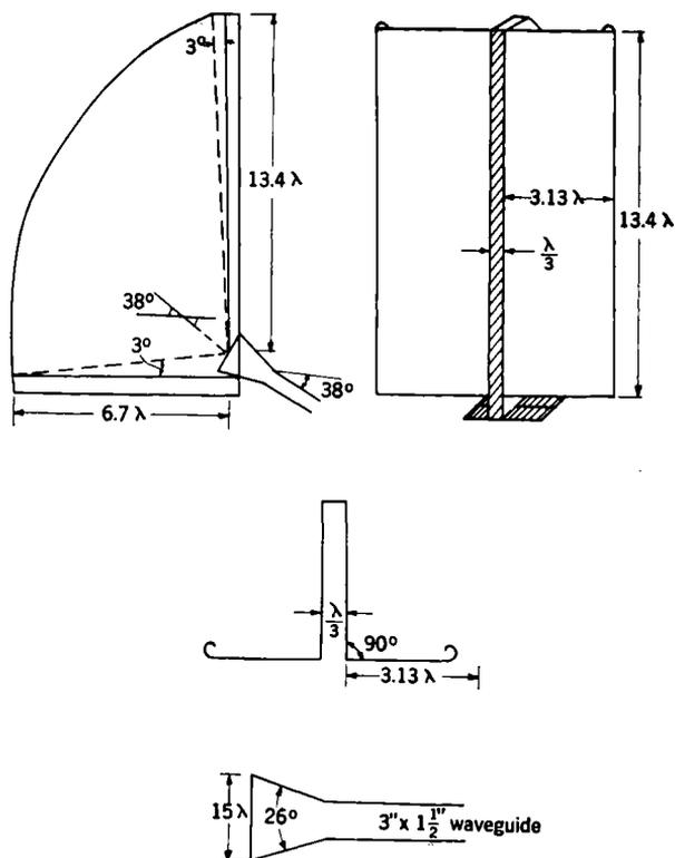
FIG. 12-27.—Half-beacon antenna.
