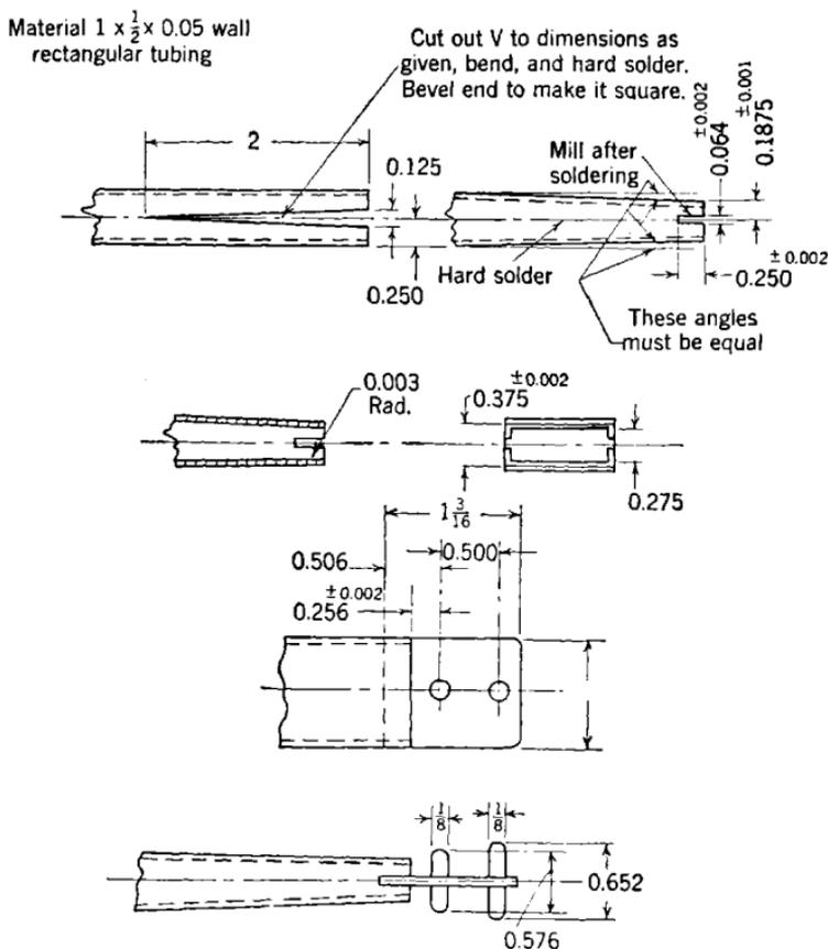
FIG. 8-14.—Waveguide double-dipole feed;  $\lambda = 3.2$  cm.
