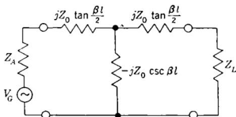
FIG. 2-10.—Circuit representation of the receiving antenna system.
