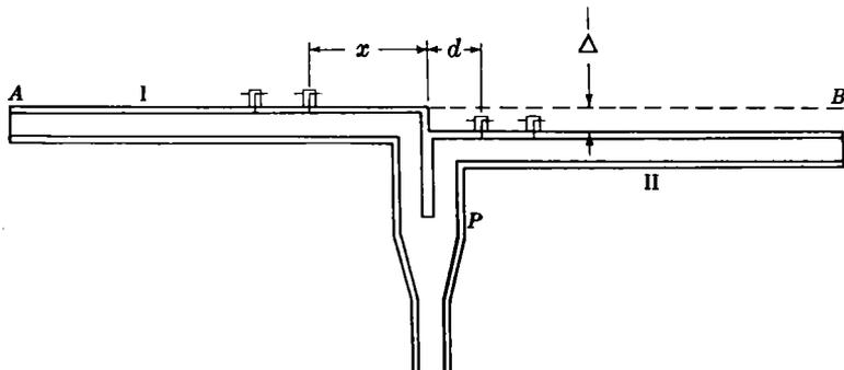
FIG. 9-58.—Schematic of broadband normal-firing resonant array system.
