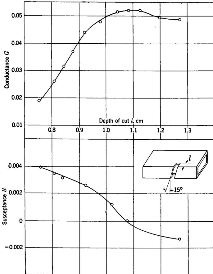
Fig. 9-22.—Admittance of a  $15^\circ$  inclined slot on narrow edge of rectangular waveguide. The waveguide dimensions are  $1\frac{1}{4}$  by  $2\frac{1}{4}$  in.,  $\lambda = 10.7$  cm., and the width of the slot is  $\frac{1}{4}$  in. (From the work of J. W. Dodds, E. W. Guphill, and W. H. Watson by permission of the National Research Council of Canada.)
