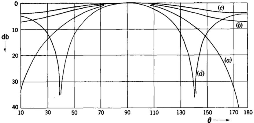
FIG. 9-8.—Array factors of four broadside arrays whose lengths are  $\lambda/2$ : (a) the two-element  $\lambda/2$ -spaced uniform array  $\cos^2\left(\frac{\pi}{2} \cos \theta\right)$ ; (b) the four-element  $\lambda/6$ -spaced uniform array
