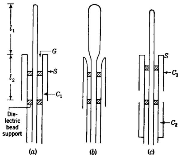
FIG. 8-1.—Skirt dipole: (a) simple form; (b) tapered gap to improve the impedance characteristics; (c) decoupling choke  $C_2$  to prevent current leakage along the outer wall.
