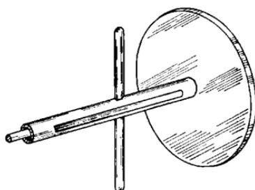
FIG. 8-12.—Dipole-disk feed.
