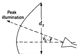
FIG. 12-21.—Offset feeding technique.
