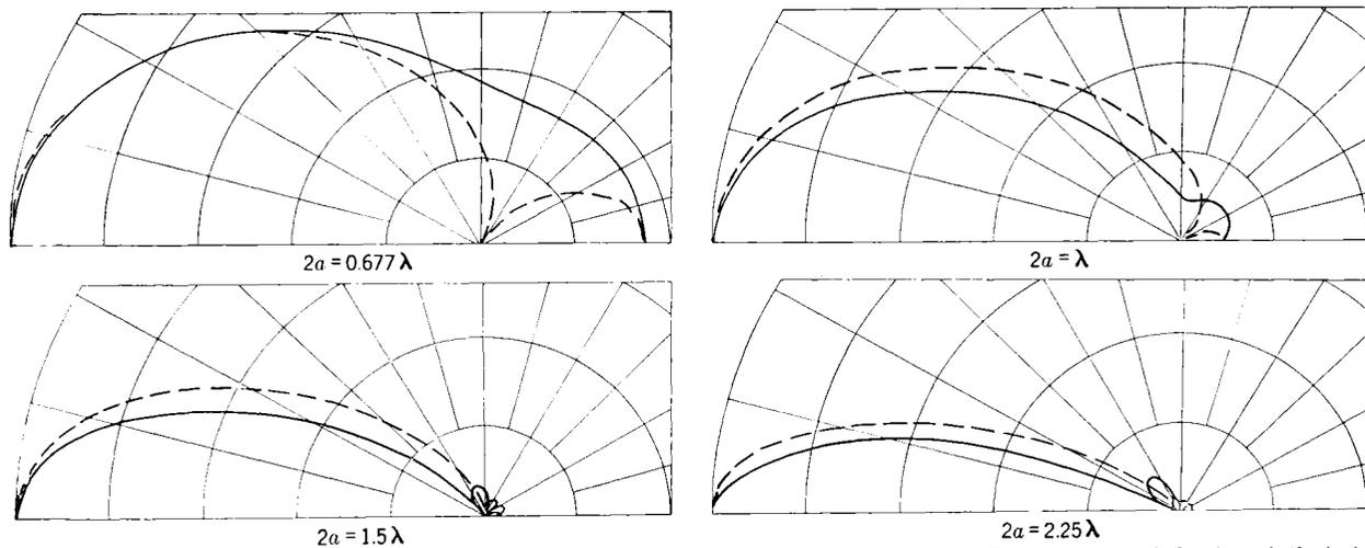
FIG. 10-2.—Circular waveguide radiation patterns for the  $TE_{11}$ -mode as a function of aperture (—  $E$ -plane; - -  $H$ -plane);  $2a$  is the inside diameter of the guide. (Courtesy of L. J. Chu and the American Institute of Physics.)
