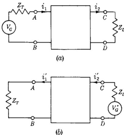
FIG. 2.3.—Reciprocity theorem for the four-terminal network.
