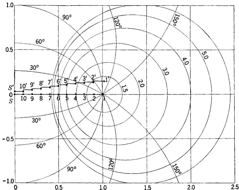
Fig. 9-48.—Input impedance of 10-element resonant array.
