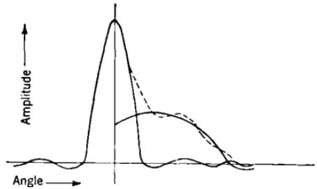
FIG. 13-32.—Superposition of barrel and paraboloidal amplitude patterns.
