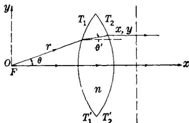
FIG. 11-6.—Coordinate system for a two-surface lens.
