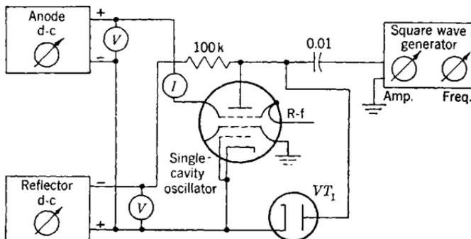
FIG. 16-1.—Diagram of a typical signal generator.
