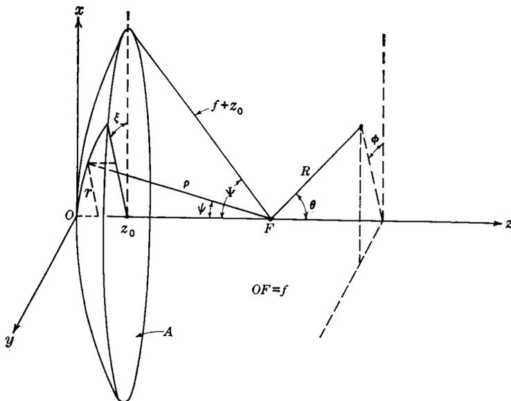
FIG. 12.1.—Geometrical parameters for the paraboloidal reflector.
