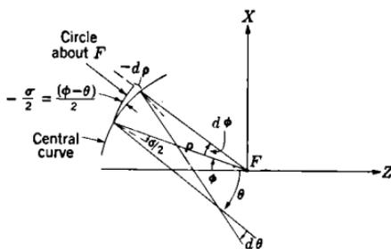
FIG. 13-35.—Geometry of central curve.
