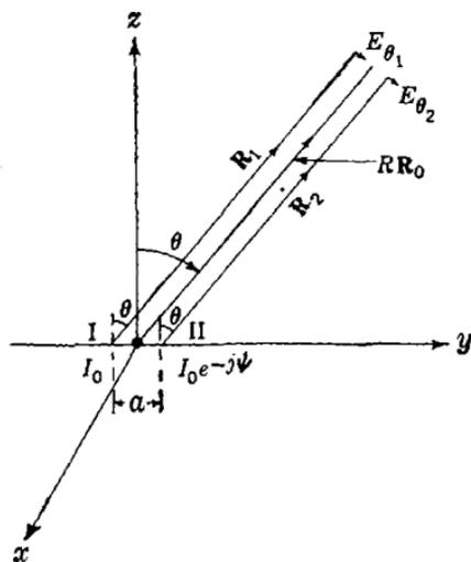
FIG. 3-14.—The double-dipole system.
