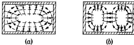
FIG. 7.10.— $TM$ -modes in rectangular waveguides: (a)  $TM_{11}$ -mode [ $\lambda_{11}^{(c)} = 2ab/\sqrt{a^2 + b^2}$ ]; (b)  $TM_{21}$ -mode [ $\lambda_{21}^{(c)} = 2ab/\sqrt{a^2 + b^2}$ ]. ——— electric field; - - - - magnetic field.
