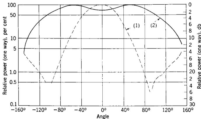
FIG. 10-31.—Primary patterns of (1) an open waveguide and (2) a cut corner waveguide ( $\phi = 63.4^\circ$  and  $C = \frac{1}{2}$ ).
