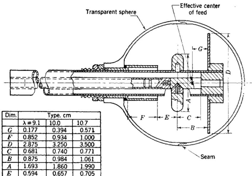
FIG. 8.10.—Dipole-disk feed assembly.
