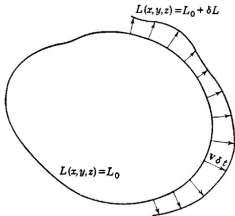
FIG. 4.2.—On the propagation of a wavefront in geometrical optics.
