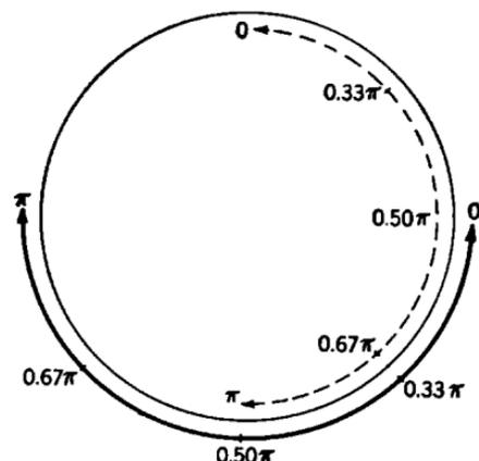
FIG. 9-4.—The range of  $\bar{z}$  due to the constant phase delay  $\psi_0 = \pi/2$  for  $s = \lambda/4$ . The dotted curve indicates the range of  $z$  associated with that of  $\bar{z}$ . The figures on the perimeter indicate the corresponding values of  $\theta$  for certain values of  $z$  and  $\bar{z}$ .
