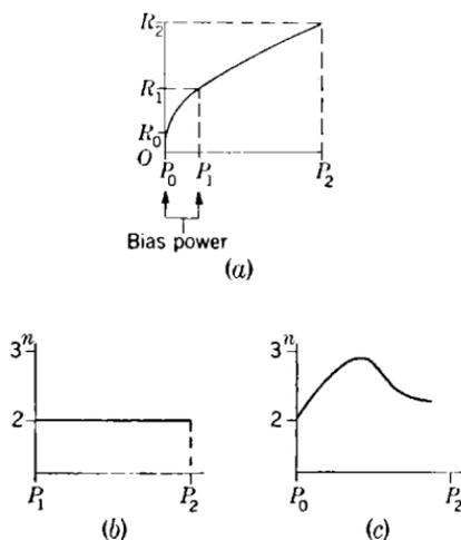
FIG. 16-8.— Characteristics of a bolometer and a silicon crystal: (a) resistance vs. power applied to bolometer; (b) "law of behavior"  $n$  vs. power above bias point; (c) "law of behavior"  $n$  vs. power for typical crystal.
