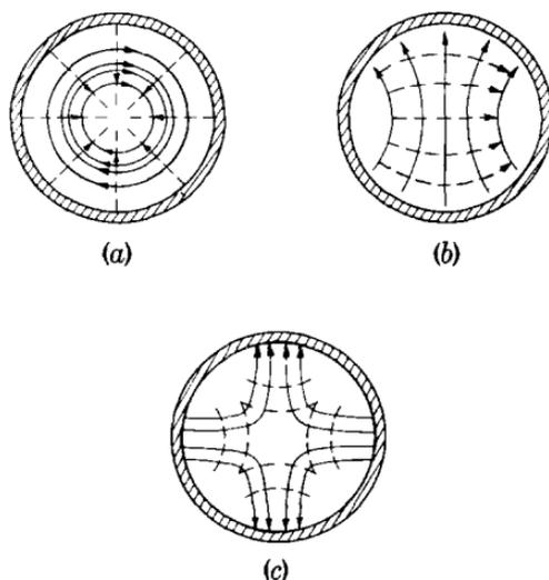
FIG. 7-14.  $TE$ -modes in circular waveguides: (a)  $TE_{01}$ -mode [ $\lambda_{01}^{(c)} = 0.82d$ ]; (b)  $TE_{11}$ -mode [ $\lambda_{11}^{(c)} = 1.71d$ ]; (c)  $TE_{21}$ -mode [ $\lambda_{21}^{(c)} = 1.03d$ ]. ——— electric field; - - - - magnetic field.
