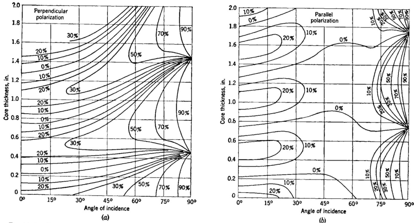
FIG. 14.17.—Typical charts showing contours of constant reflection as a function of core thickness and angle of incidence for the following conditions:  $\lambda_0 = 3.2$  cm; core  $\epsilon'/\epsilon_0 = 1.4$ ; skin  $\epsilon'/\epsilon_0 = 3.7$ ; skin thickness = 0.050 in. (a) Polarization perpendicular to the plane of incidence; (b) parallel polarization.
