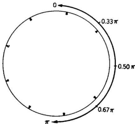
FIG. 9-3.—The location of the zeros of  $f(z) = 1 + z + z^2 + \dots + z^8$ . The range of  $z$  for  $s = \lambda/4$  is also shown together with a few of the corresponding values of  $\theta$ .
