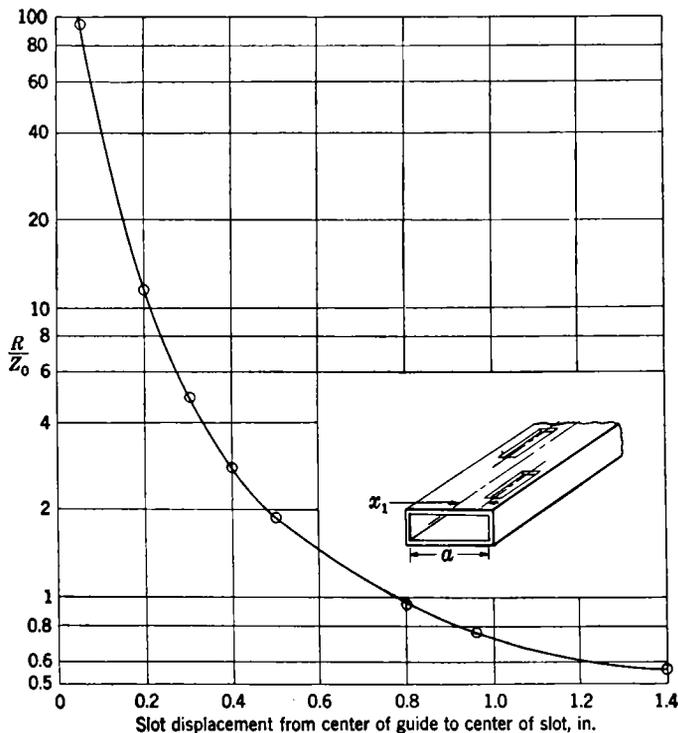
FIG. 9-18.—Resistance offered by a longitudinal slot as a function of its displacement from the center. The slot dimensions are  $\frac{1}{8}$  by 2 in., the waveguide is  $1\frac{1}{2}$  by 3 in.,  $\lambda = 10.7$  cm. The data fit the relation  $G = Z_0/R = 1.73 \sin^2 [(\pi x/a)1]$ . (From J. W. Dodds, E. W. Guptill, and W. H. Watson by permission of the National Research Council of Canada.)
