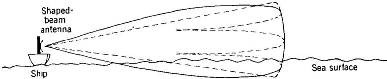
FIG. 13-3.—Sector shaped beam for surface search by shipborne antenna.
