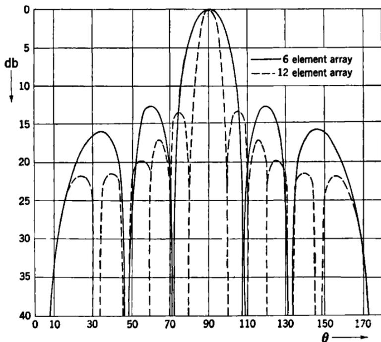
FIG. 9-6.—Graphs of  $\frac{\left[ \sin^2 \left( \frac{n\pi}{2} \cos \theta \right) \right]}{\left[ n^2 \sin^2 \left( \frac{\pi}{2} \cos \theta \right) \right]}$  for  $n = 6$  (full curve) and  $n = 12$  (dotted curve).
