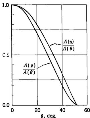
FIG. 11-3.— $A(\rho)/A(\theta)$  for a spherical lens and  $A(y)/A(\theta)$  for a cylindrical lens with hyperbolic contours;  $n = 1.6$ .
