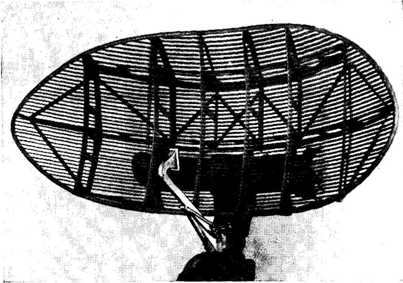
FIG. 12-23.—Fanned-beam antenna using the offset feed technique.
