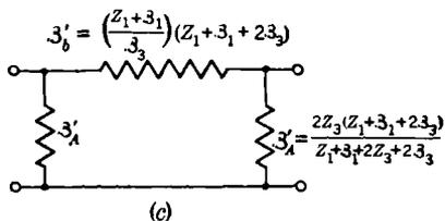
FIG. 9-42.—Network system equivalent to a loaded transmission line: (a) T-section replacements of radiators and line segments; (b) reduction to symmetrical networks; (c)  $\Pi$ -section equivalent of the network in (b).
