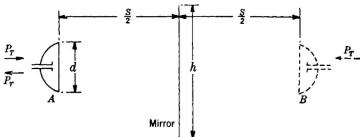
FIG. 15-18.—On the reflection method for gain determination.
