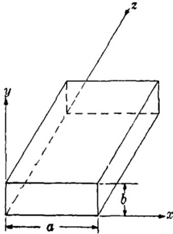
FIG. 7-8.—Rectangular waveguide.
