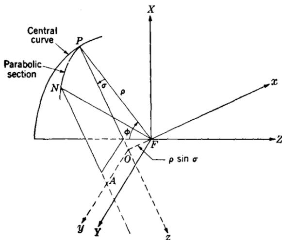
FIG. 13-34.—Surfaces of parabolic section.
