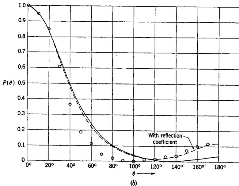
FIG. 10-4.—Theoretical and observed radiation patterns from rectangular waveguide;  $\lambda = 3.2$  cm;  $\frac{a}{\lambda} = 0.71$ ;  $\frac{b}{\lambda} = 0.32$ ; ——— calculated patterns;  $\circ$  observed values; (a) *E*-plane; (b) *H*-plane.
