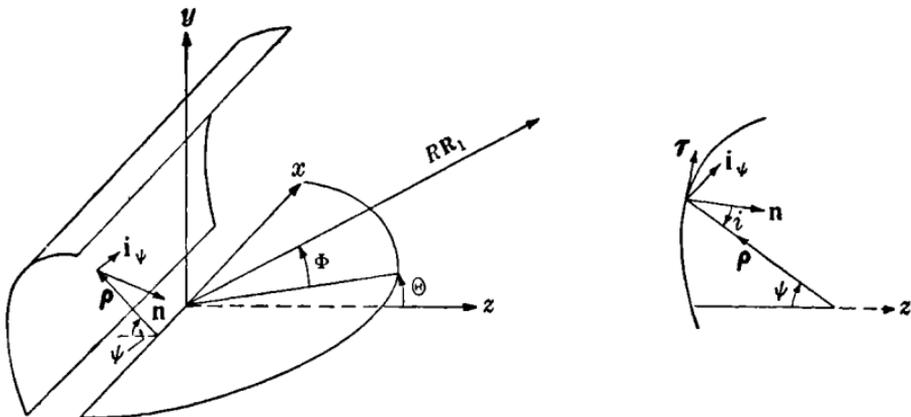
Fig. 5-9.—The cylindrical reflector with a line-source feed.
