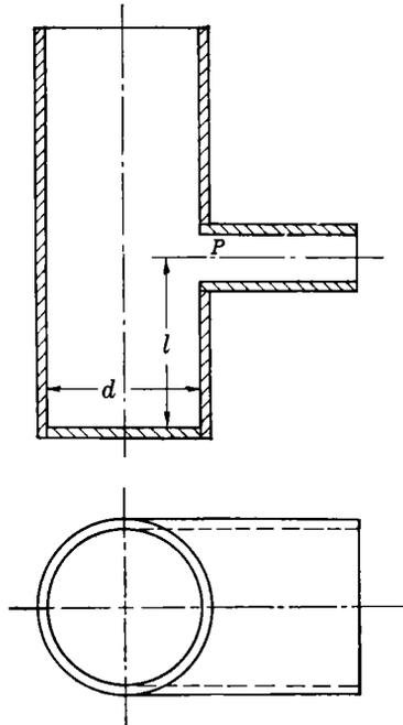
FIG. 9-33.— $TE_{10}$ - to  $TM_{01}$ -mode converter.
