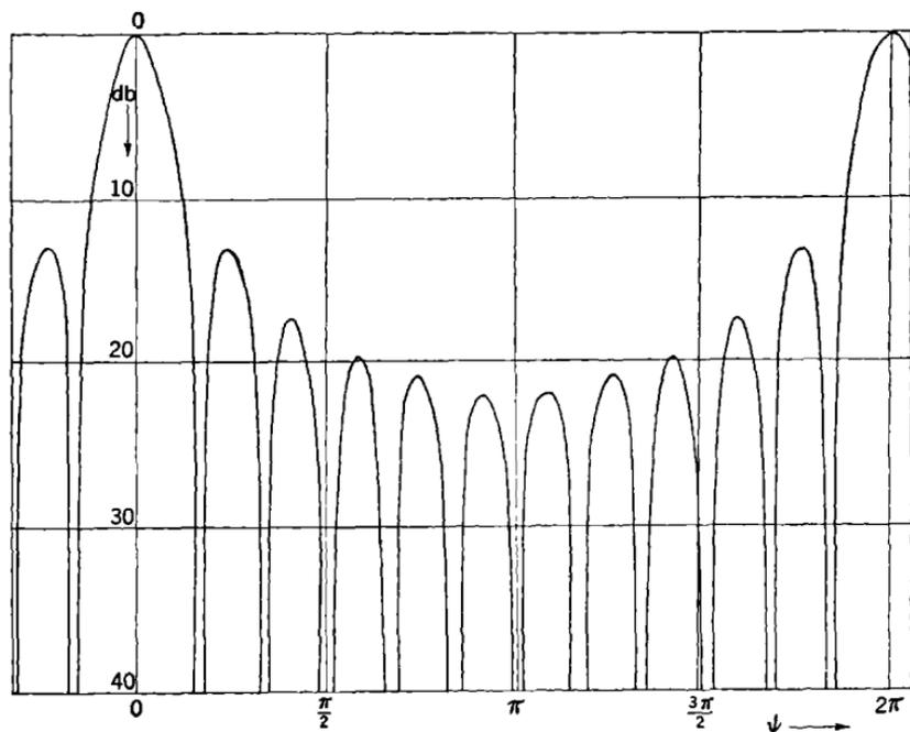
FIG. 9-5.—The function  $\frac{\left(\sin^2 \frac{n}{2} \psi\right)}{\left(n^2 \sin^2 \frac{1}{2} \psi\right)}$  for  $n = 12$ .
