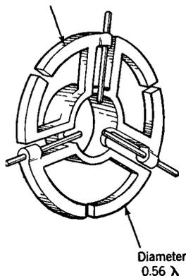
FIG. 9-28.—Tridipole radiator.
