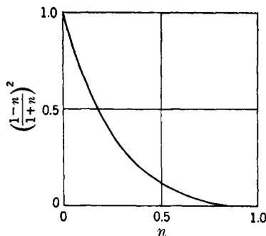
Fig. 11-19.—Power reflection at normal incidence as a function of  $n$ .
