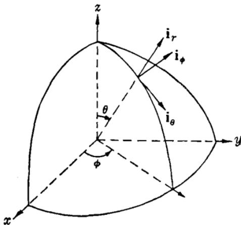
FIG. 3-3.—Spherical coordinates.
