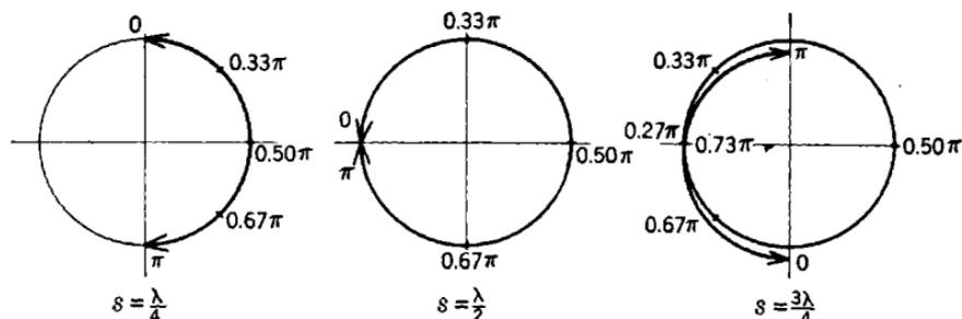
FIG. 9-2.—The portion of the unit circle in the complex plane that is the range of  $z$ . The real axis is horizontal. The figures on the perimeter show the corresponding values of  $\theta$  for certain values of  $z$ .
