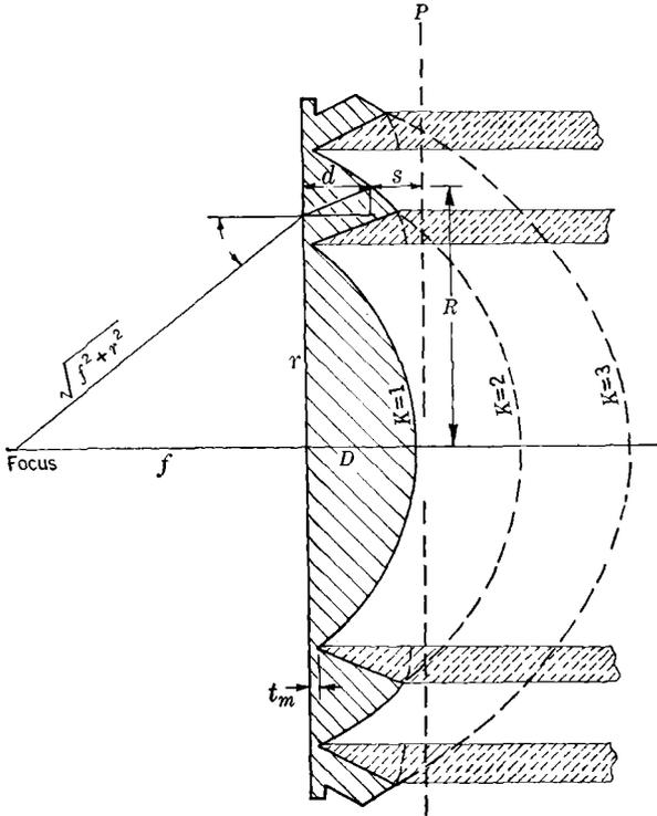
FIG. 11-8.—Zoned two-surface lens.
